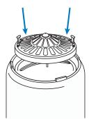
2. Reattach top tank snap ring. Pull up on the top cap to seat the O-rings.
