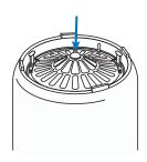
3. Release the red button and inspect the system for leaks. After inspecting for leaks, allow water to run through the system for 10 minutes for the final flushing period.
