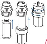
Press new replacement filter to the top of the filter housing using the appropriate color coded filters. Then, reconnect the bottom of the filter housing to the top half. Ensure the threads are correctly aligned, then turn clockwise to tighten. Continue this step for the second and third filter housing.
