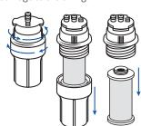
**NOTE:** If filter housing is too tight to disconnect by hand, please use the plastic wrench included with original system.
