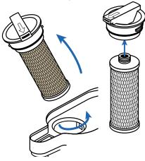
2. Press new filter into filter chamber cap ensuring a snug fit. Insert into housing unit and twist right to close.
