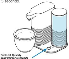
5. While red light is illuminated, press and hold dock button for 1 second. Light will blink red. While system flushes, light will continue to
