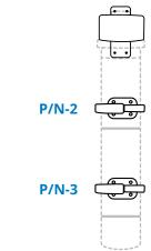
D. Place cartridge into brackets and connect to system head by turning to the right.
