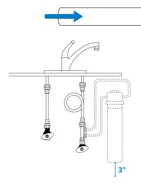
Three (3) inches of clearance from the base of the filter is needed for easy cartridge replacement.
