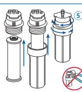
Reattach filter housings to the bottom of the system manifold. Ensure connection points are correctly aligned, then push the filter housing up while turning to the right. Turn until you feel a 'click' and the filter housing is locked into place. Continue this step for the second and third filter housing. Ensure all filter housings are locked into place, are not on an angle, and are aligned as pictured. Improper placement may result in damage to the o-ring or leakage.
