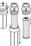
**NOTE:** If filter housing is too tight to disconnect by hand, please use the plastic wrench included with original system.
